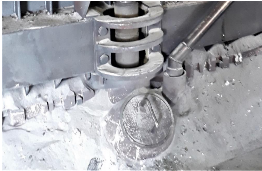
Figure 13. Final revised alumina chute implemented at CBA Soderberg cells.
